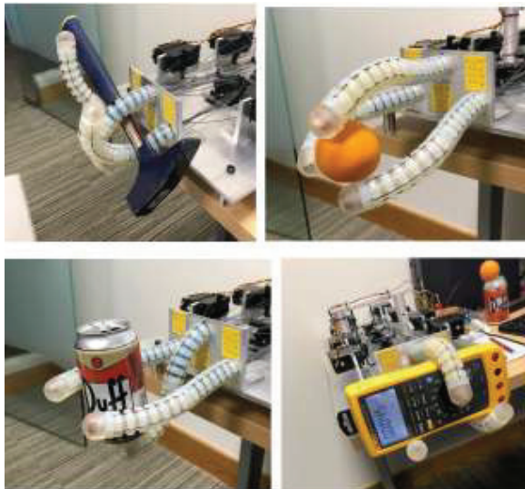
Illustration 8: The Cthulhu-Morphic Gripper grasping common tools and laboratory supplies.
