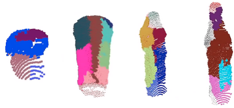
Fig. 2. Supervoxels computed on identified clusters in point clouds of sample objects (including an apple, paper cup, water bottle, and oil bottle) where different colors indicate supervoxels in the cluster. Uncolored or gray regions represent the small sized clusters which are considered to be a part of the same smooth surfaces and were not processed for the supervoxel computation.
