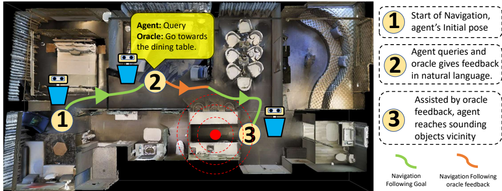
Figure 1: An illustration of our proposed AVLEN framework. The embodied agent starts navigating from location denoted ① guided by the audio-visual event at ③. At location ②, the learned policy for the agent decides to seek help from an oracle (e.g., because the audio stopped). The oracle provides a short natural language instruction for the agent to follow. The agent translates this instruction to produce a series of navigable steps to move towards the goal ③.
