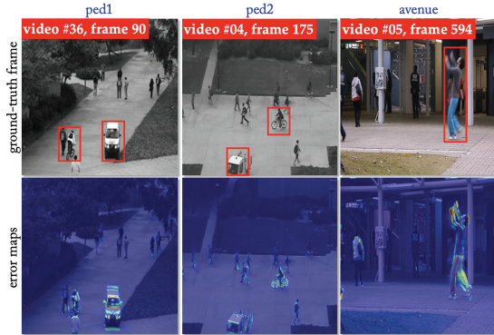
Figure 6: Difference maps. We show examples of cross-domain frame prediction comparison on three datasets (source: SHT). The lighter colors in difference map mean larger prediction error indicating anomalies. Red boxes indicate ground truth anomalies. Best viewed in color.
