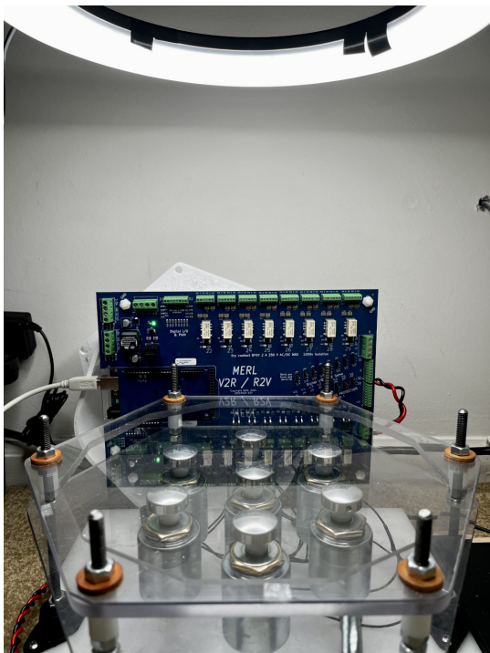
Fig. 1: The 7-solenoid impact manipulation system "Thumper"; the seven solenoids beneath a transparent support surface are in the foreground, with the controller board in the background
