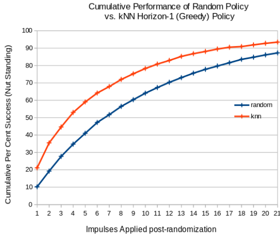
Fig. 15: Cumulative success rates of the benchmark random policy and the self-supervised kNN policy
