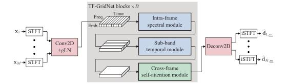
Figure 2: Overview of TF-GridNet. Here, gLN stands for global layer normalization.
