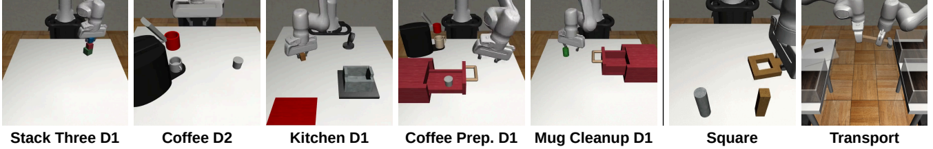
Fig. 3: Evaluation tasks from the Robomimic and MimicGen benchmarks. (The Stack D1 task uses two cubes, while Stack Three D1 uses three).
