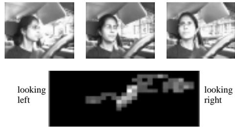
Figure 7: At top, three sample images from a driving sequence. At bottom, the pose-space histogram for this sequence, showing a peak for the driver looking straight-forward, and side lobes corresponding to viewing the side and rear-view mirrors.
