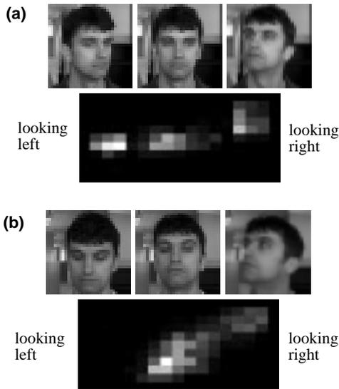
Figure 6: **(a)** The images show the three head poses adopted repeatedly over an extended sequence, together with the pose-space histogram which shows three distinct peaks for those head poses. **(b)** A similar experiment but two of the head poses (forward and forward-down) are not sufficiently far apart to register as distinct peaks in the pose-space histogram.
