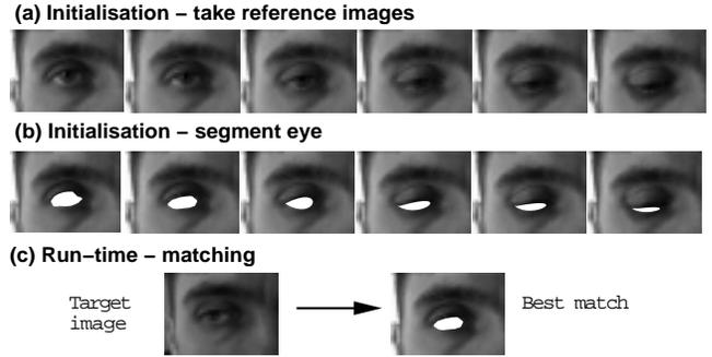
Figure 3: *(a)* a series of reference images of the eye is taken at initialisation time, *(b)* semi-automatic processing is performed to segment out the interior of the eye, resulting in a set of templates which are used for matching at run-time, *(c)* a target image of the eye is processed to find the best-matching template; the iris in the target image has moved, which would degrade the template matching if it were included in the processing.
