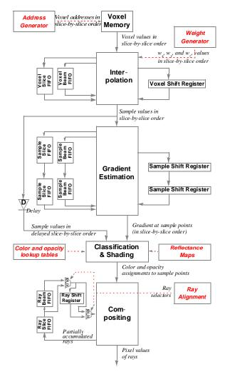
Figure 3: Conceptual ray-casting pipeline.
