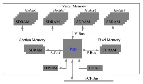
Figure 14: VolumePro PCI board diagram.
