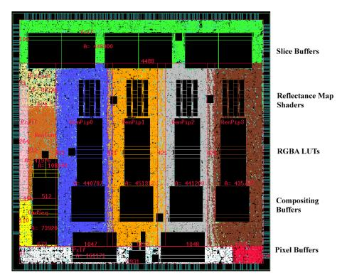
Figure 11: Layout of the vg500 ASIC with four vertical rendering pipelines. Captions on right refer to SRAM blocks in the image.
