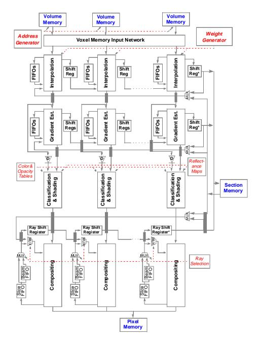
Figure 12: The four parallel pipelines of the vg500 ASIC. Modules shown in blue are off-chip memory.
