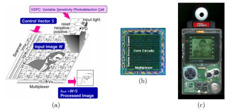
**Figure 3:** Some real-time applications can be made faster using specialized hardware. A CMOS detector made by Mitsubishi Electric, called the artificial retina chip, can both detect the image and perform some image processing operations, (a). (b) shows the chip. The Nintendo GameBoy Camera uses the artificial retina chip and allows the player's face to be inserted into a simple game. The retina chip is used for both detection and image enhancement.
